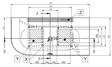
Product measure tolerances ± 10 mm Frame location tolerance according to  $X \pm 20 \text{ mm}$
