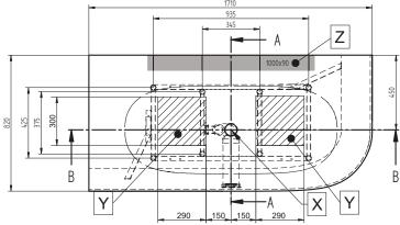
Product measure tolerances  $\pm$  10 mm Frame location tolerance according to X  $\pm$  20 mm
